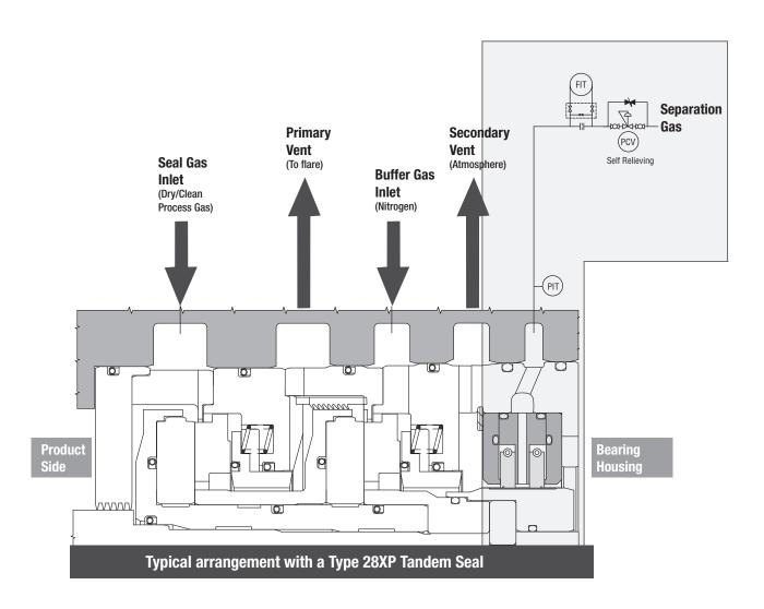
Separation gas can be pressure controlled (recommended, to minimise gas consumption) or flow controlled. Typical example shown, variations may be necessary depending on individual circumstances including availability and quality of separation gas and safety considerations.
