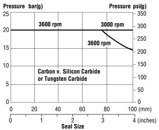
To determine the maximum pressure for the size of Type 515E seal required, multiply the pressure obtained from the chart by the appropriate factors given in chart below.
