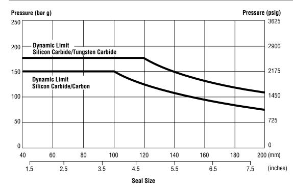
The basic pressure rating is for a standard seal, as shown in the typical arrangement, when installed according to the criteria given in this data sheet and generally accepted industrial practices.
