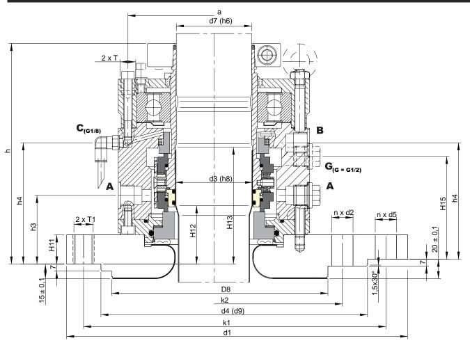
**CK736** CK736 D Dry running, easy barrier gas supply Liquid lubricated with dry nitrogen
