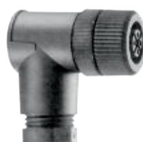
The GEMÜ 1219 is a connector (cable socket / cable plug) M12, 5-pin. Straight and/or 90° angled plug type. Defined cable length or with threaded connection without cable. Various materials available for the fixing nut.
