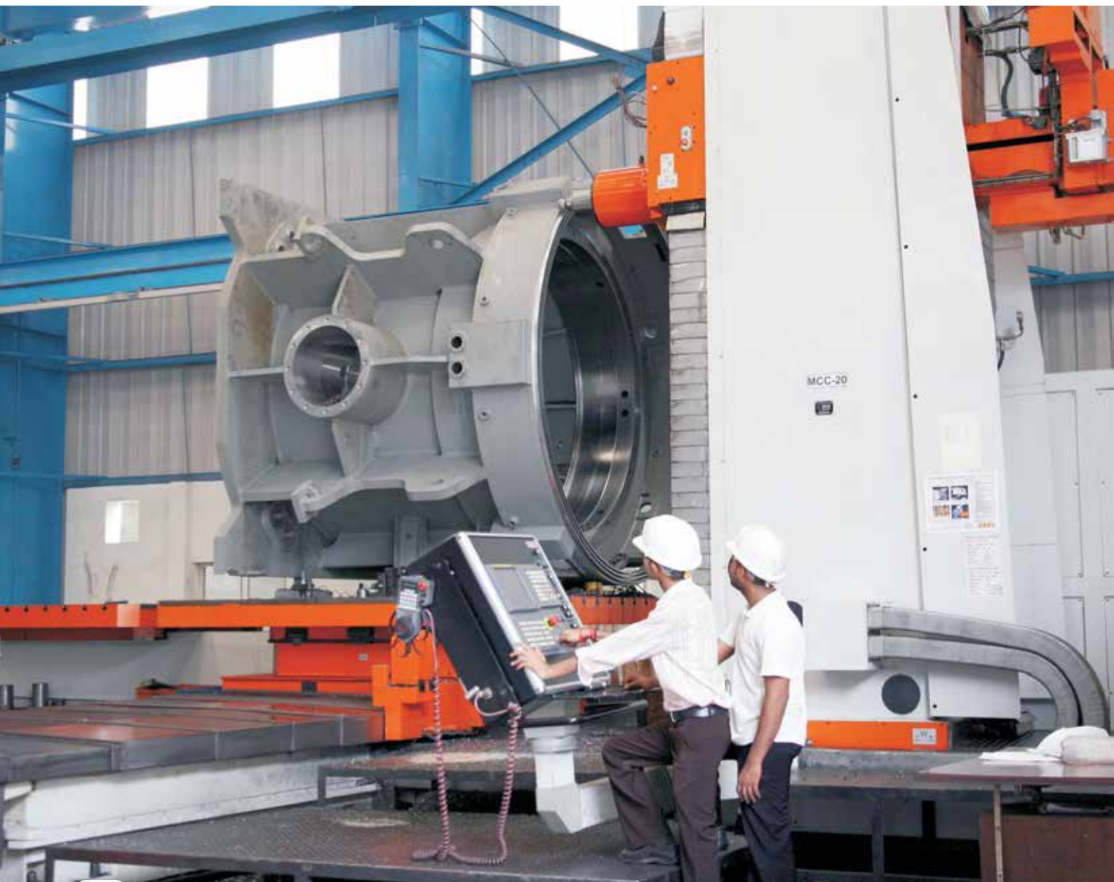
(Bevel-Planetary gear box casing under machining on CNC Horizontal machine center)
