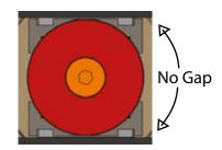
Our innovative Zero Backlash mechanism improves performance and solves the wearing-related gap issues between the sliding block and the scotch yoke slot, maintaining friction at similar levels to even the most established technology. It is available on request, please contact us for more information.
