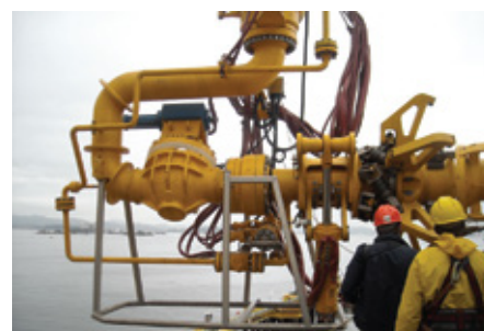
Our Top Entry Ball Valve is fully integrated into the high pressure unloading arm for LNG Floating Storage Regasification Unit in Brazil's Guanabara Bay LNG Terminal
